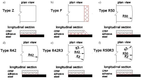
Fig. 2. Schematic of strip end shapes
