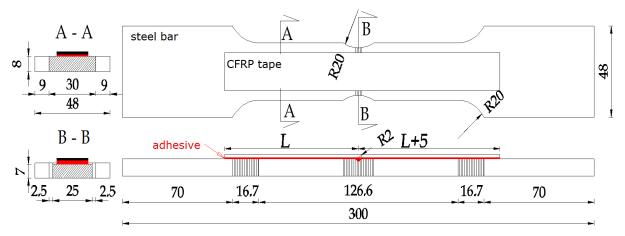
Fig. 1. Schematic design of the test sample
